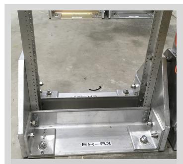
Shake-table tests identified the need to strengthen existing aluminum racks to limit swaying.
