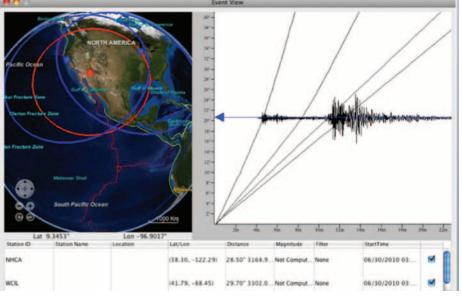
**Figure 5.** Students can use jAmaseis software to record data from any global sensor available via IRIS Data Services or from their own educational seismograph and then can calculate earthquake locations using that data (http://www.iris.edu/hq/inclass/software-web-app/\_jamaseis).
