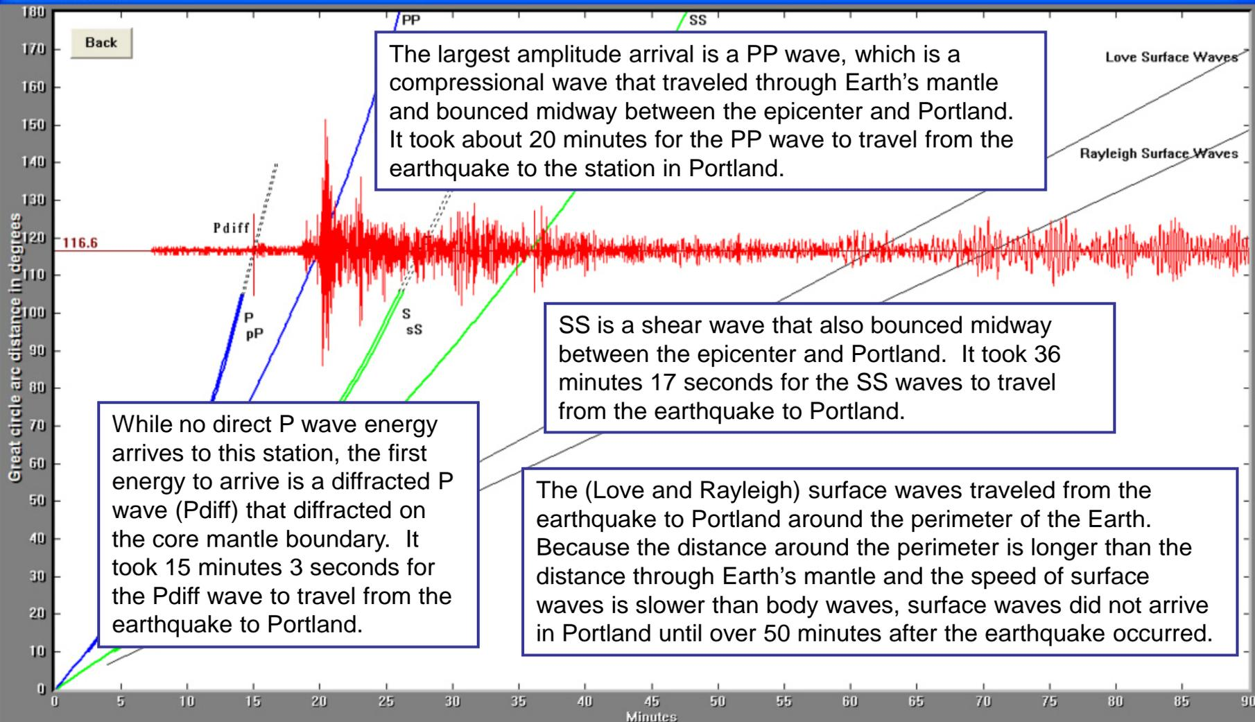
The largest amplitude arrival is a PP wave, which is a compressional wave that traveled through Earth's mantle and bounced midway between the epicenter and Portland. It took about 20 minutes for the PP wave to travel from the earthquake to the station in Portland.
