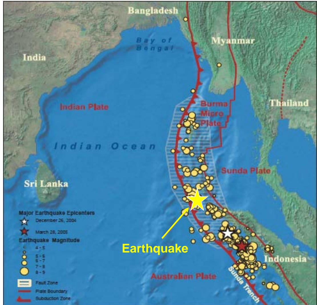
Map showing the earthquake epicenter, aftershocks, and the extent of the main fault rupture for the M 9.1 December 26, 2004 earthquake (white) and the M 8.7 March 28, 2005 earthquake (red).
