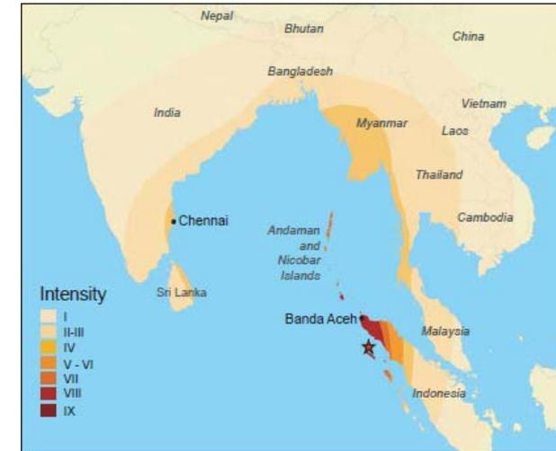
Modified Mercalli Intensity (MMI) map of the M 9.1 2004 earthquake, showing violent shaking and heavy damage (MMI level IX) on the western coast of Aceh Province of Indonesia.
