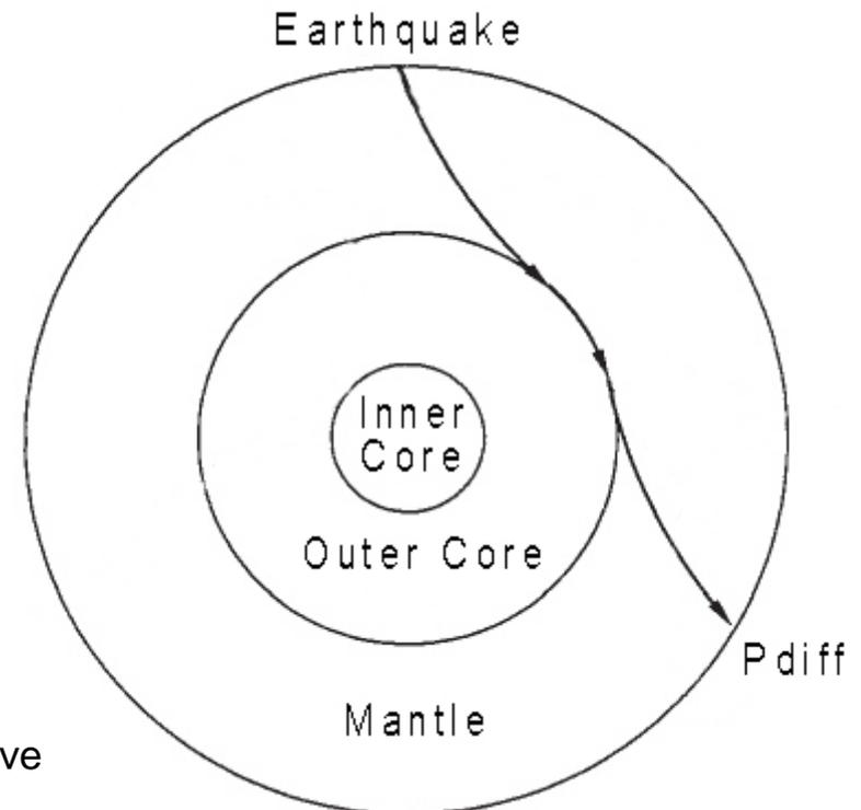
Travel path of the diffracted P wave
