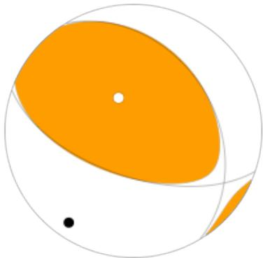
Shaded areas show quadrants of the focal sphere in which the P-wave first-motions are away from the source, and unshaded areas show quadrants in which the P-wave first-motions are toward the source. The dots represent the axis of maximum compressional strain (in black, called the "P-axis") and the axis of maximum extensional strain (in white, called the "T-axis") resulting from the earthquake.
