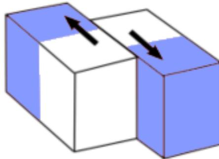
The offset direction of a strike-slip fault is the direction a feature is displaced when you cross the fault. The road is displaced to the right, so this is a “right-lateral” strike-slip fault.
