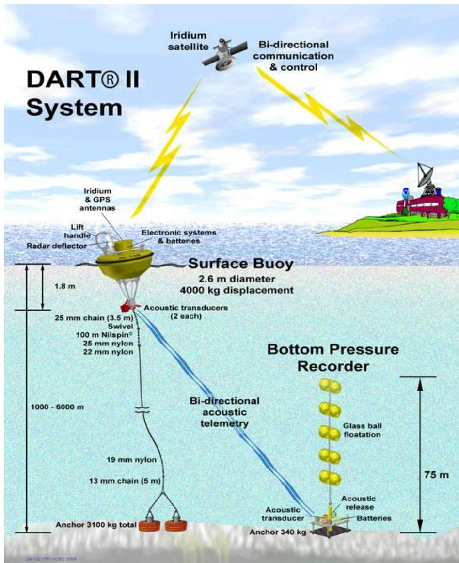
The DART II® system consists of a seafloor bottom pressure recording (BPR) system capable of detecting tsunamis as small as 1 cm, and a moored surface buoy for real-time communications.
