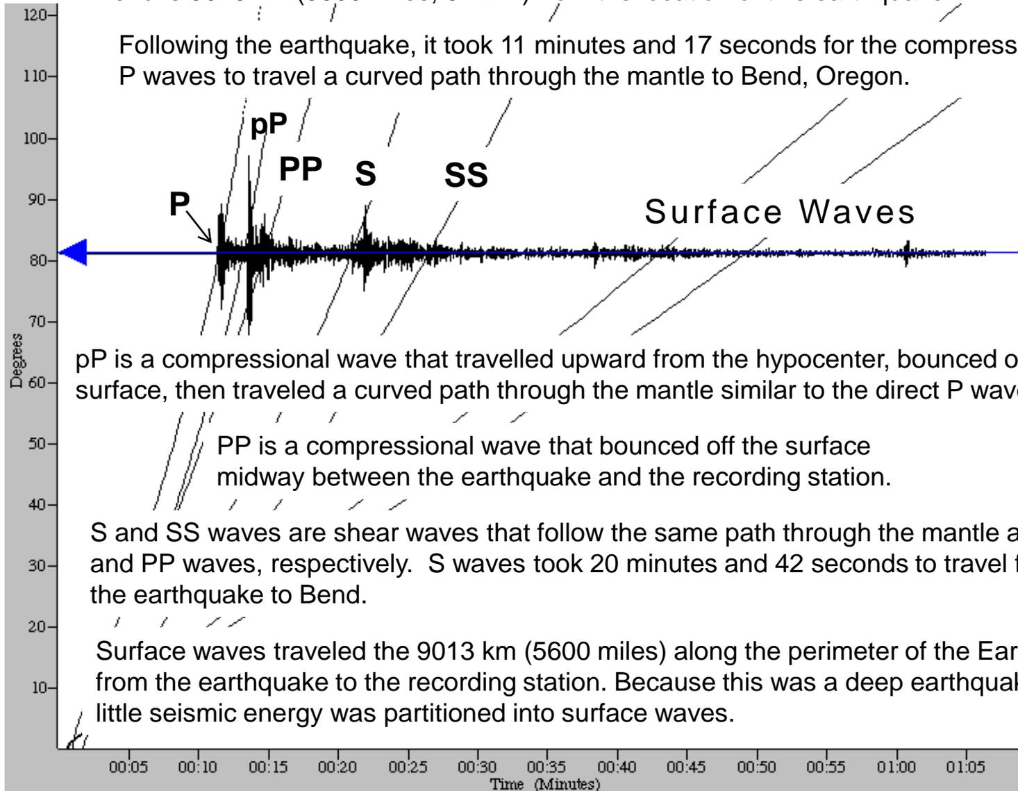
pP is a compressional wave that travelled upward from the hypocenter, bounced off the surface, then traveled a curved path through the mantle similar to the direct P wave.
