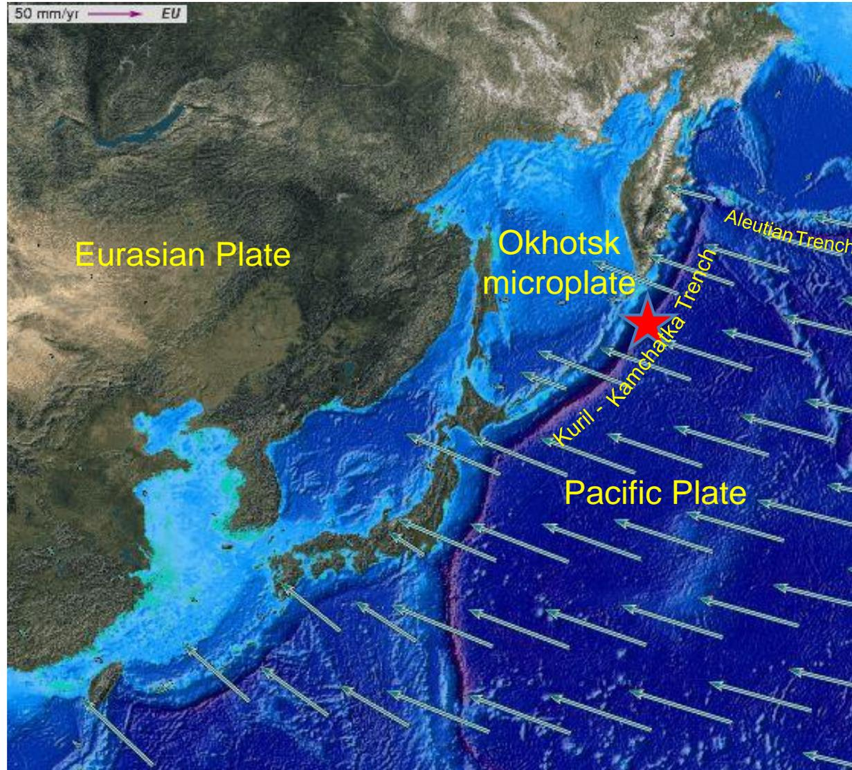
The map on the right shows regional seismicity along the Kuril-Kamchatka Trench. Earthquake depths in the Kuril-Kamchatka subduction zone increase from southeast to northwest as the Pacific Plate dives deeper beneath the Okhotsk microplate.
