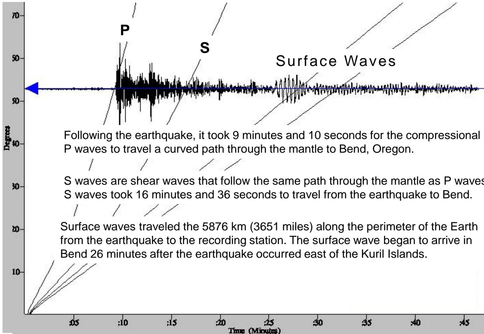
Following the earthquake, it took 9 minutes and 10 seconds for the compressional P waves to travel a curved path through the mantle to Bend, Oregon.
