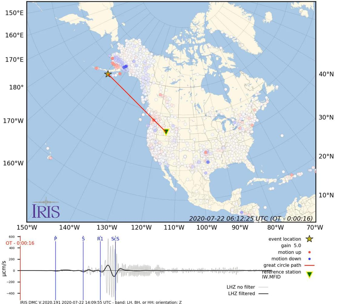
Seismic waves crossing the US recorded by the USArray.
