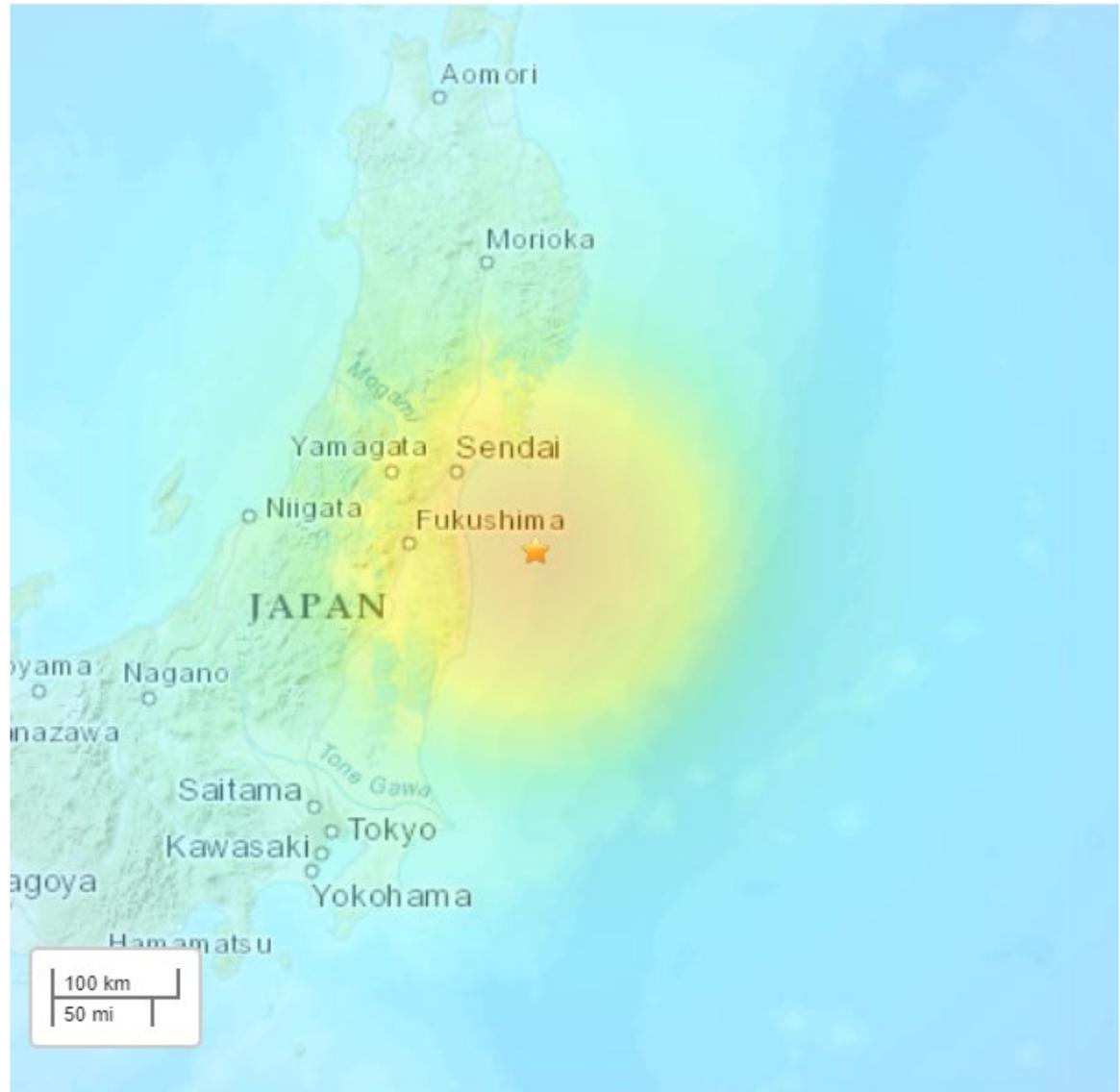
*USGS estimated shaking intensity from M 7.3 Earthquake*
