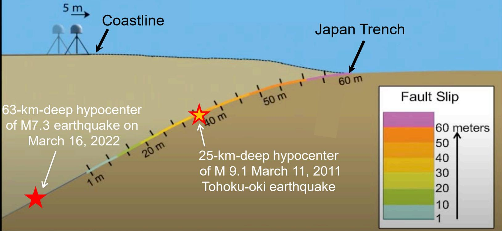
Fault slip during the M 9.1 Tohoku-oki earthquake is shown on this cross section through its hypocenter at ~25 km depth. Fault slip was 40 meters at the hypocenter and over 60 meters at the Japan Trench. Fault slip decreased downdip from the hypocenter to about 1 meter at ~50 km depth. The hypocenter of March 16, 2022 M 7.3 earthquake projects into this cross section at or just beyond the downdip limit of the 2011 rupture.
