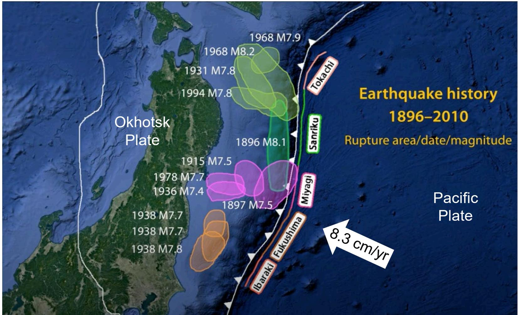
On this map, the year, magnitude, and rupture area are shown for magnitude 7.4 and larger earthquakes on the Pacific – Okhotsk subduction plate boundary from 1896 to 2010, just prior to the March 11, 2011 magnitude 9.1 great earthquake.
