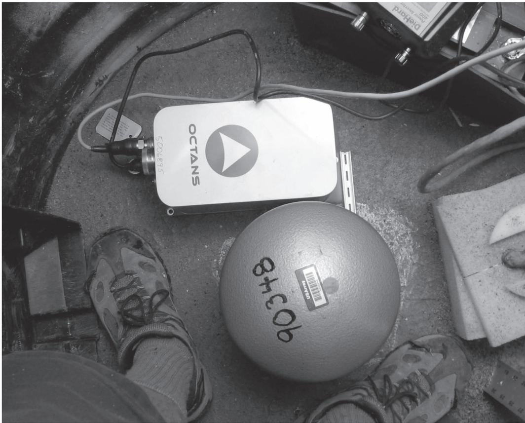
▲ **Figure 6.** Octans device aligned with an STS-2 within a TA station vault. The small size and insensitivity to magnetic influences of this device are key advantages for performing in-situ measurements of sensors. The device determines orientation with respect to the rotation axis of the Earth within 10 minutes. (Photo: R. W. Busby.)
