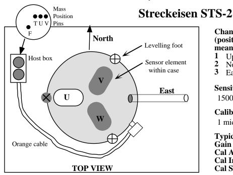
**Channel Order** (positive voltage on DAS channel means ground moved in given direction)
