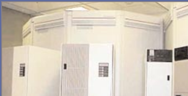
StorageTek Mass Storage System. The new DMC Mass Storage System can hold 6000 tapes, each with a capacity of 60 gigabytes. The system presently has 9T-9940 high performance tape drives with an aggregate input/output rate of nearly 100 megabytes/second. (Photo courtesy of NCAR)
