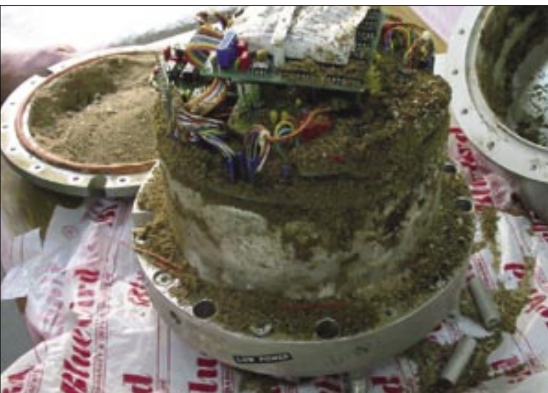
Ouch! An STS-2 seismometer fully packed with sand by diligent termites.
