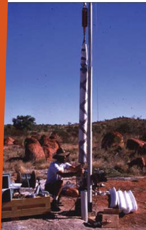
WRAB - IDA engineer Todd Johnson lowers a KS-54000 into a borehole at GSN station WRAB (Warramunga, Australia).
