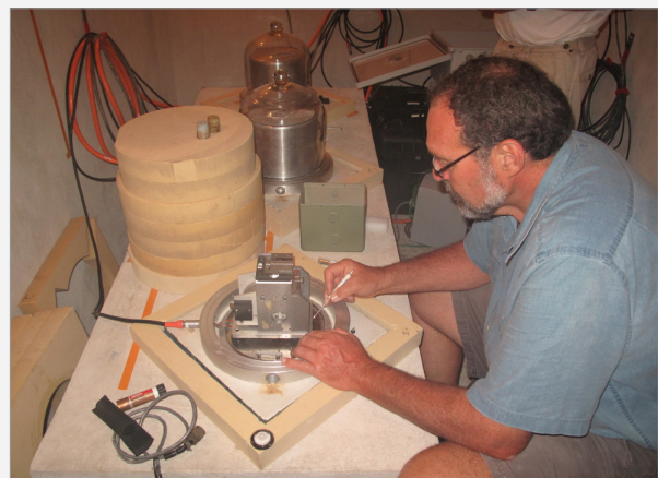
IDA engineer David Chavez adjusts an STS1 seismometer at station JTS (Las Juntas, Costa Rica). The station's pier was rebuilt and a recording building replaced during a major renovation this year.
