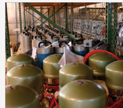
Seismometers at the PASSCAL Instrument Center prior to deployment.
