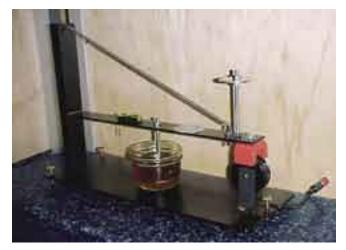
The AS-1 is an affordable seismometer that is robust enough to be operated in high schools and that transparently demonstrates seismometry principles.
