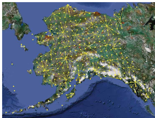
Figure TA-6. Hub-and-spoke deployment strategy for Alaska. Each hub is at a location accessible by road or large aircraft. The ends of the spokes are station locations.
