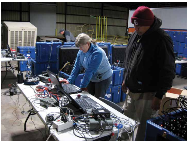
Figure PS-4. PASSCAL field engineers programming Texan recorders for the Salton Seismic Imaging Project, 2011.
