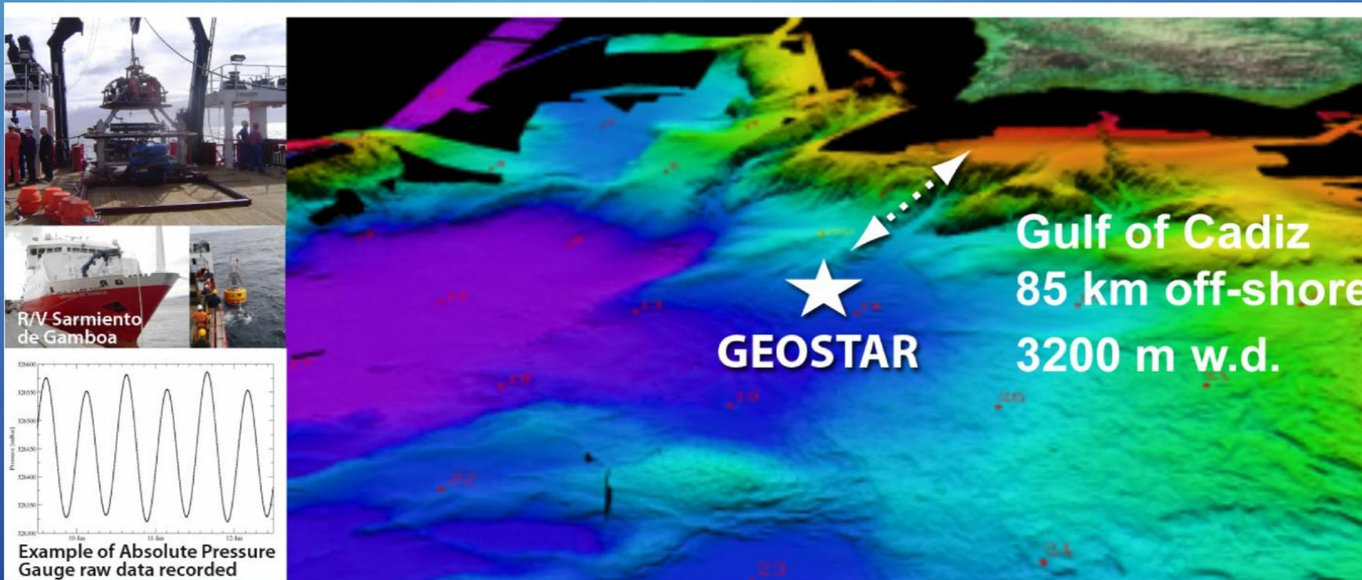
**INFRASTRUCTURE GEOSTAR** observatory, seafloor station with acoustic connection to a surface buoy and satellite connection from buoy to shore.
