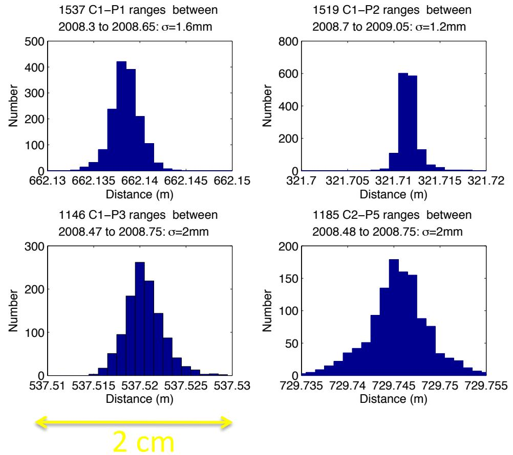
~1 mm/yr interseismic strain signals are detectable over 1-5 km baselines.
