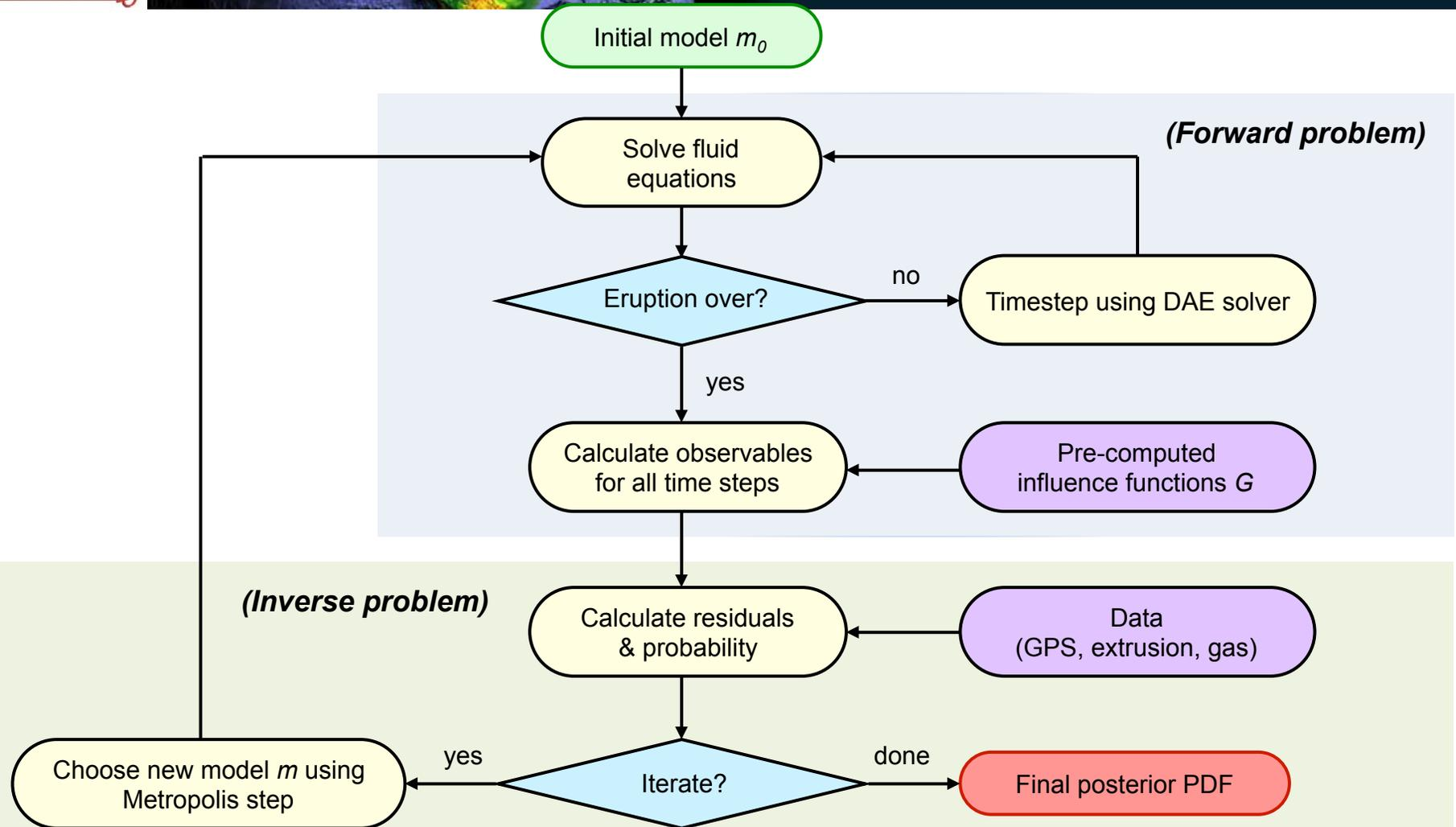
$$P(\mathbf{d}_1, \mathbf{d}_2, \dots, \mathbf{d}_K | \mathbf{m}) = \prod_{k=1}^K \left\{ (2\pi\gamma_k^2)^{-N_k/2} |\Sigma_k|^{-1/2} \exp\left(-\frac{1}{2\gamma_k^2} \mathbf{r}_k^T \Sigma_k^{-1} \mathbf{r}_k\right) \right\}$$
