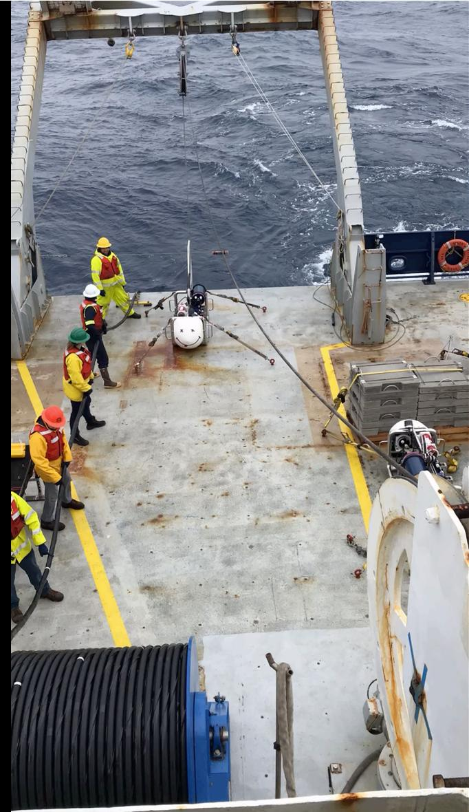
Step 2: deploy, deep-tow, & nav Scripps transmitter
