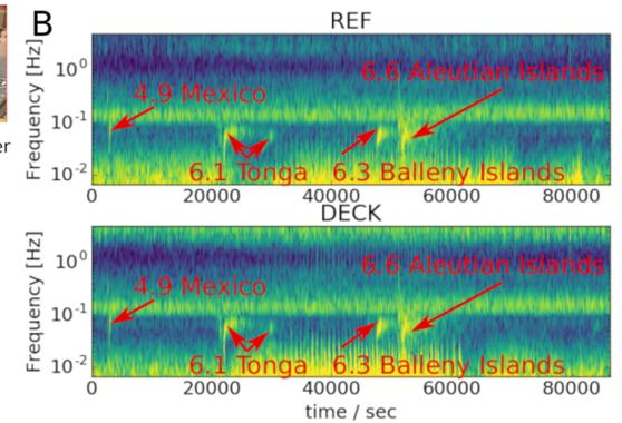
On deck operation on MSL engineering model shows clean recording of teleseismic events and simple transfer function from ground motion. Air motion causes decoherence. Lander activity not considered here (measurements were taken over a weekend, and engineering model does not require active thermal management used on Mars).
